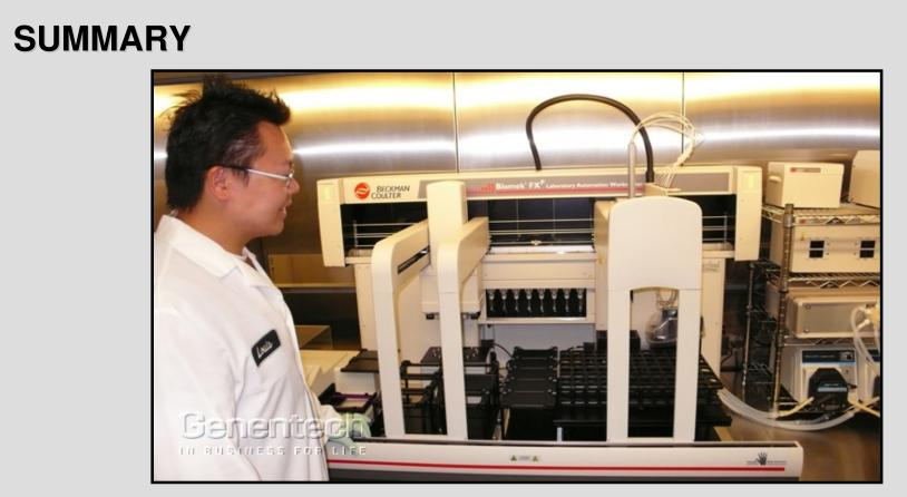
Successfully developed a high-throughput system for cell culture (HTS-CC) with  $\geq$ 10x throughput compared to manual operation: • Current maximal throughput: 384 samples (4 x 96 samples)
